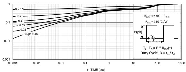
11. Normalized Thermal Transient Junction to Ambient
