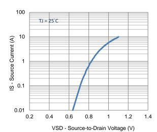
4. Drain-to-Source Forward Voltage
