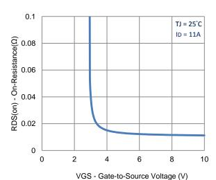
3. On-Resistance vs. Gate-to-Source Voltage
