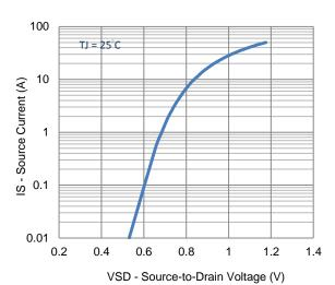
4. Drain-to-Source Forward Voltage
