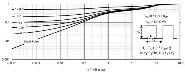
11. Normalized Thermal Transient Junction to Ambient
