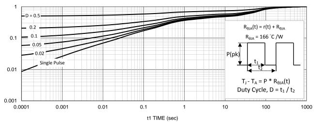
11. Normalized Thermal Transient Junction to Ambient
