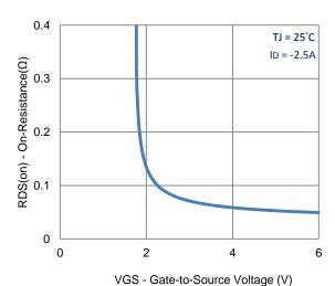
3. On-Resistance vs. Gate-to-Source Voltage
