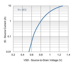
4. Drain-to-Source Forward Voltage
